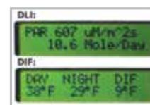
Displays Daily Light Integral (DLI) and Day/Night Temperature Difference on the LCD
