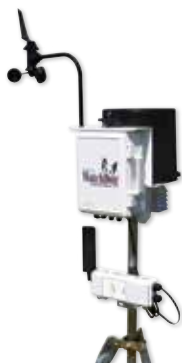
3923 DataScout Modem mounted with a WatchDog 2000 Series Full Weather Station
